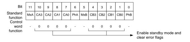
Programming current value "0000" for both coils at a time clears the overcurrent flags and switches the TMC236 into a low current standby mode with coils switched off.
